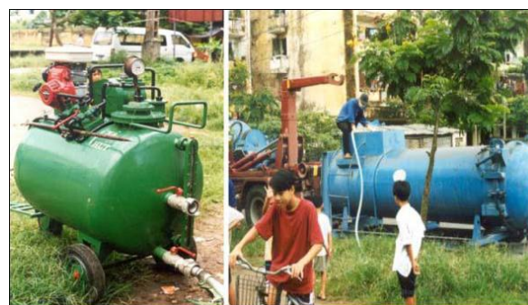
Figure 4-50. 0.35 m 3 manual desludging truck and supporting 10m 3 intermediate tanker
