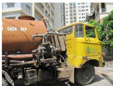
Figure 4-25. Truck with separate vacuum pump at work
