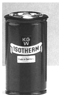
Figure 14. One of the Dewar vessels used for laboratory-scale experiments on thermal composting.
