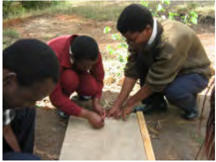
The door frame is made with wooden “brandering” and triangular plywood corners. A single diagonal strut supports the frame. Some form of covering is added to the frame. In this case sacking material called hessian.
