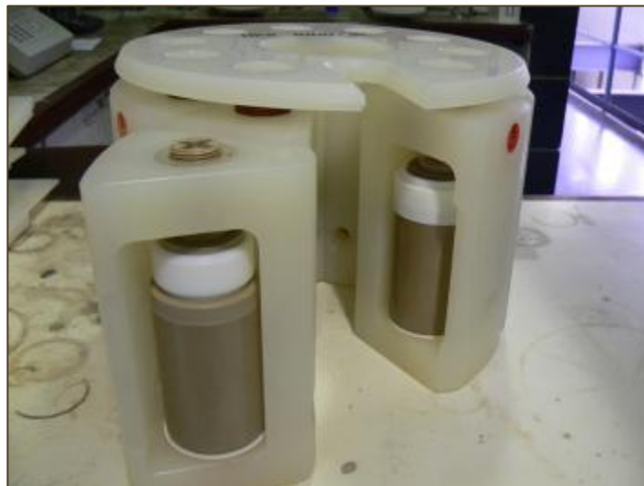
High Performance Microwave Digestion System (ETOS One)
