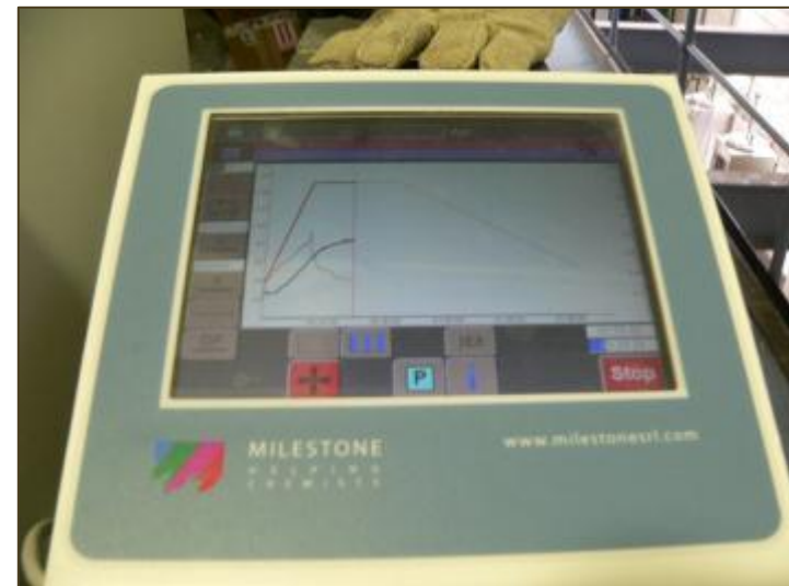
High Performance Microwave Digestion System (ETOS One)
