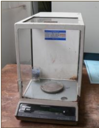
Fine Balance (Mettler AE 160)
