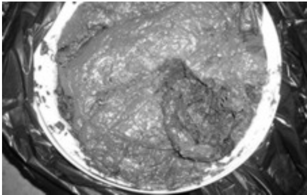
Pit latrine contents sampled from the top layer of a primary school pit latrine. This sample contains mostly faecal material.
