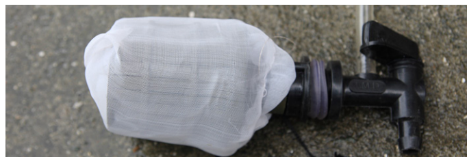
Figure 6: Tap with filter and level tube.
