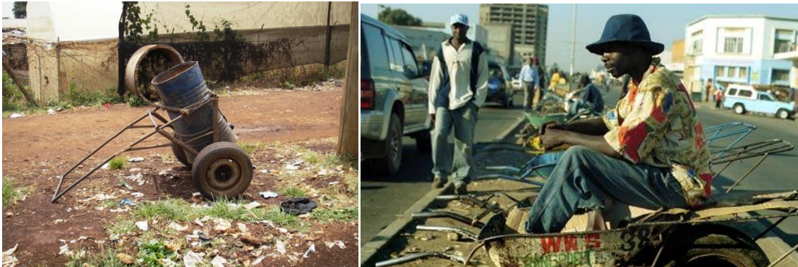
Figure 3: Left: Showing a heavily used cart in Nairobi. Plastic sheet is sealed over the top of the drums with a rubber tie or rope to stop its contents from sloshing out. Right: Common wheel barrow used in Kanyama
