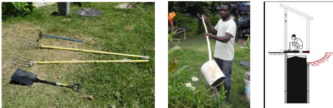
Figure 2: Left Gardening tools for pit emptying; Middle: Dipper for more liquid content; Right: Access to pit latrine
