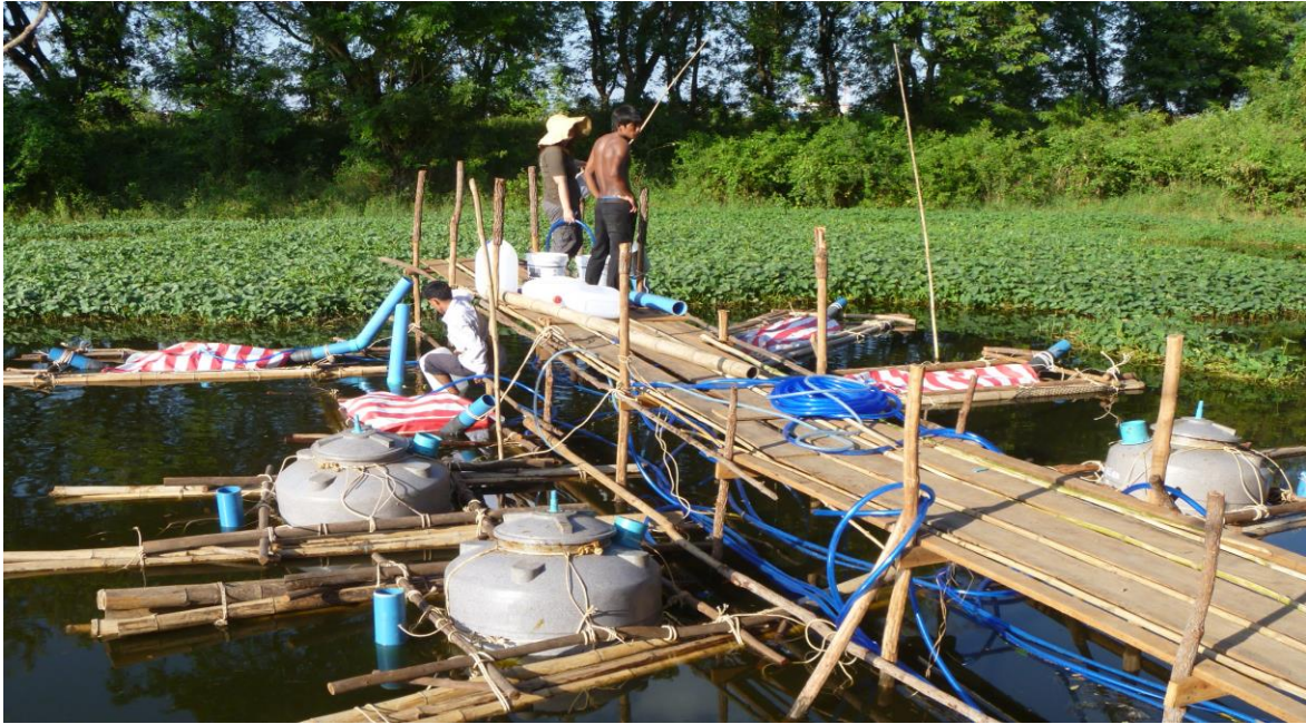
Figure 22. Experimental setup of the biodigesters at Royal University of Agriculture in Phnom Penh.
