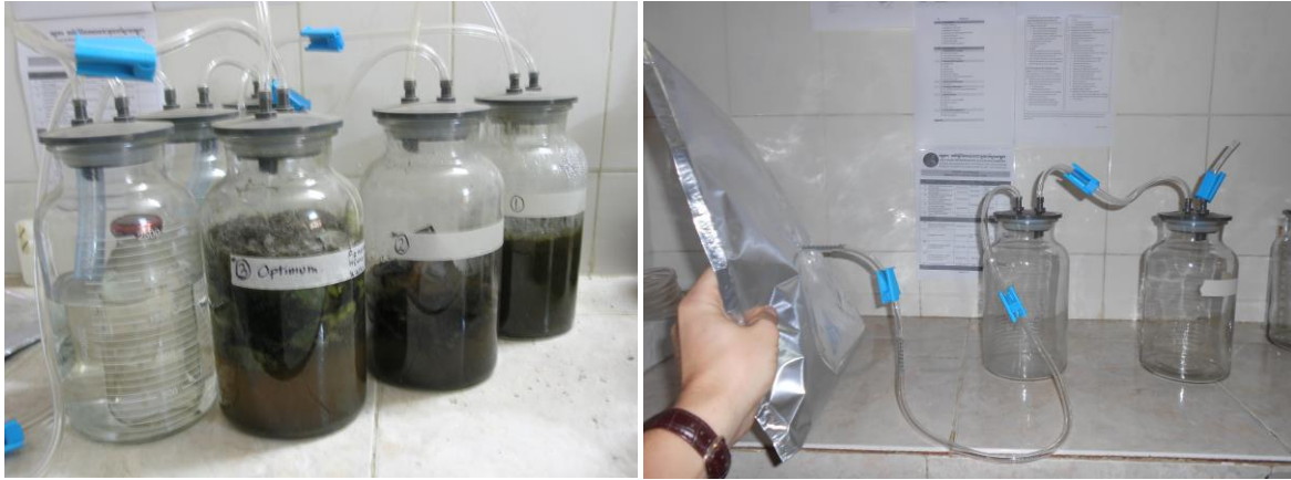
Figure 37. Setup of the lab scale anaerobic digestion. The right cylinder in the left picture consists of the substrate and the left cylinder of 3M NaOH. The blue clamps closes the hoses when necessary to stop the flow. The gasbag is located in the right picture.
