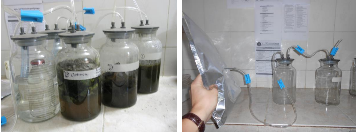
Figure 21. Setup of the lab scale anaerobic digestion. The right cylinder in the left picture consists of the substrate and the left cylinder of 3M NaOH. The blue clamps straps the hoses when necessary to stop the flow. The gasbag is located in the right picture.
