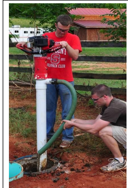
Fig 1. Initial prototype being tested on mixture of bentonite and horse manure.
