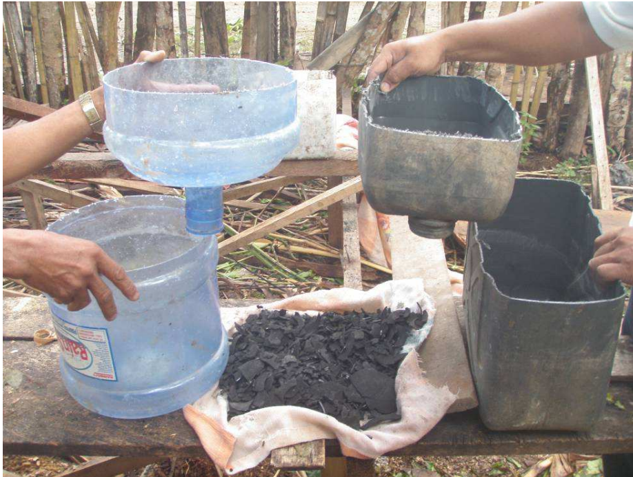
Photo 6. Basic materials for urine collector. The charcoal is used to prevent smell and to contain N escaping to the atmosphere.
