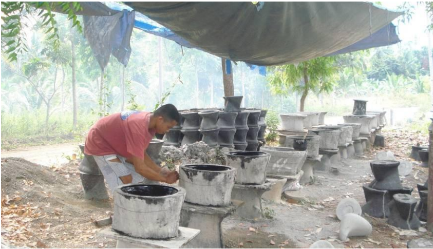
Photo 5: Ecosan toilet bowl production site in Libertad, Misamis Oriental. The production area is located in a 6-hectare farm demo area of the WAND Foundation.
