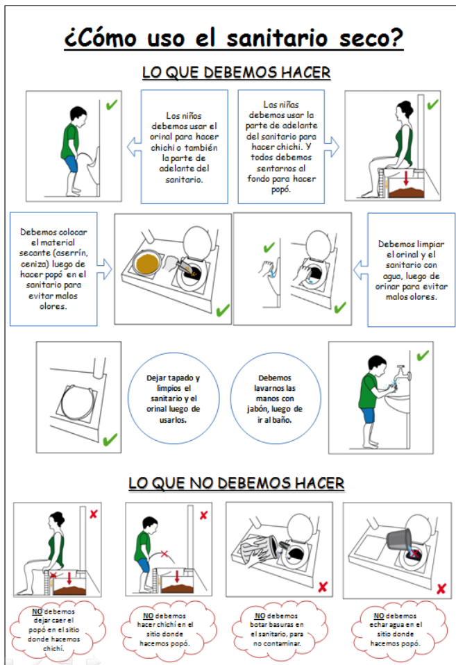
Fig. 14: Poster describing adequate use of UDDTs. The pictures are adapted from: http://www.rotaria.net/peru3/rotaria/files/DL_7_Man.jpg
