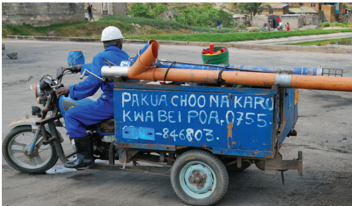
Fecal sludge management in dense, unplanned neighborhoods is well suited to local micro-enterprises, such as this one, which uses a specially designed handpump and a motorized tricycle fitted with a small tank to provide desludging services in Dar Es Salaam, Tanzania.
