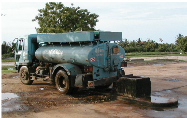
A vacuum truck at a dumping site managed by the Municipality of Dar es Salaam, Tanzania. Photograph © Hydroconseil
