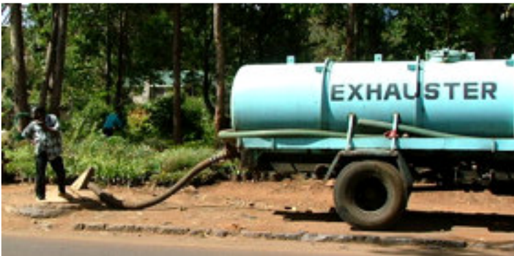
Transfer into sewers is permitted in Nairobi (but not Dar or Maputo) (© Linda Tyers)
