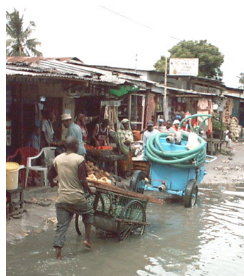
A Vacutug (specialised pit-emptying machine) on the way to the treatment works, Dar es Salaam (© David Schaub-Jones)
