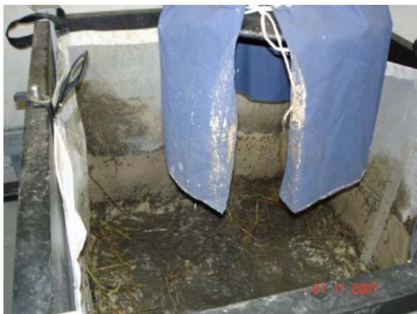
Fig. 11: Compost filter bags at trial stage, here with straw as structure material (source: LINZ AG, November 2007).
