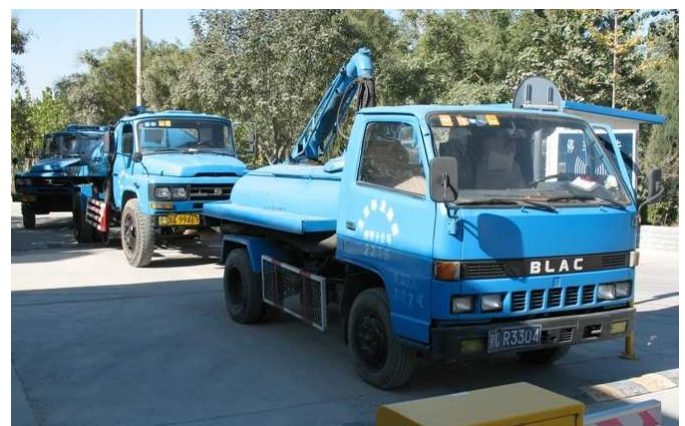
Fig. 7: Type of vacuum trucks to be used for the transport of scum and sludge from the septic tanks at the public toilet blocks with low flush, urine diverting toilets in the Olympic Forest Park. This picture was taken at an MBR wastewater treatment in metropolitan Beijing.
