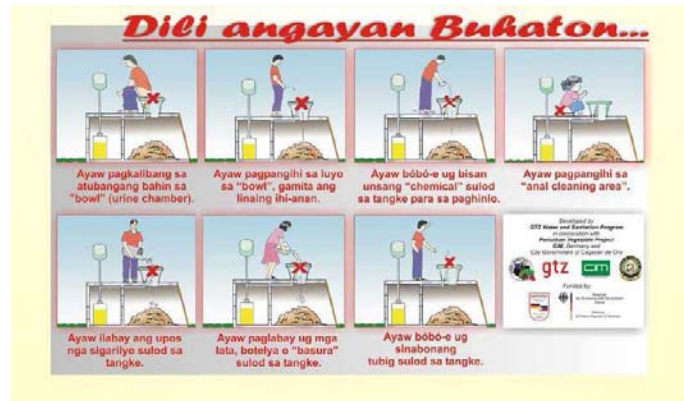
Fig. 15-b: User guidelines "Don'ts" for UDD toilets (source: DILG-GTZ Water & Sanitation Program Philippines, 2006).
