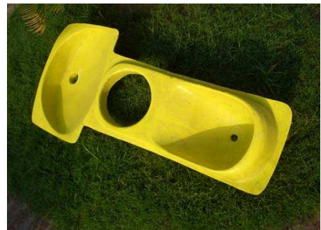
Fig. 10: Urine-diversion squatting pan that allows separate collection of urine, faeces and anal washwater (source: seecon GmbH, which year? Supplier?). The anal washwater section on the left of the pan was found to be too small.
