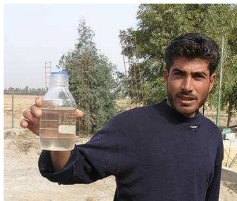
Fig. 3: Operator at treatment plant, showing effluent quality of constructed wetland when plant had been operational for 8 years (source: E. v. Münch, Jan. 2009)
