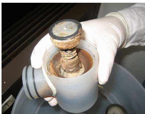
Fig. 9: Soft urine precipitations inside a urine valve of a Roediger urine-diversion toilet. This valve was disassembled and cleaned after clogging (source: L. Ulrich, December 2008). One valve costs EUR 118 and requires a bowden cable costing EUR 51(location of valve in Fig. 7).
