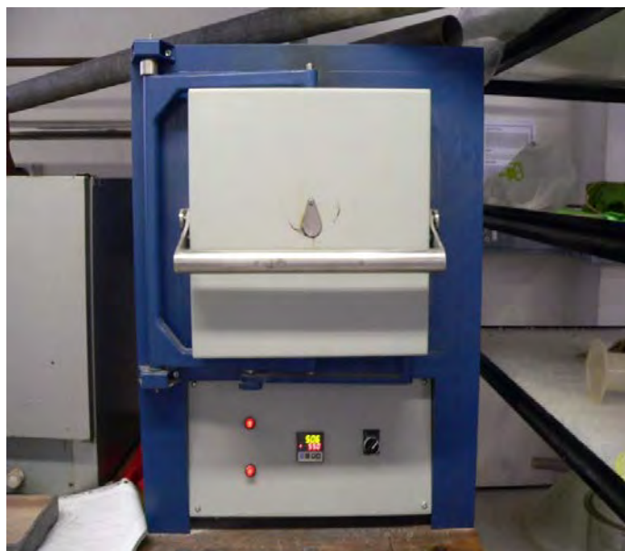
Furnace (E160) - Temperature: 550 °C
