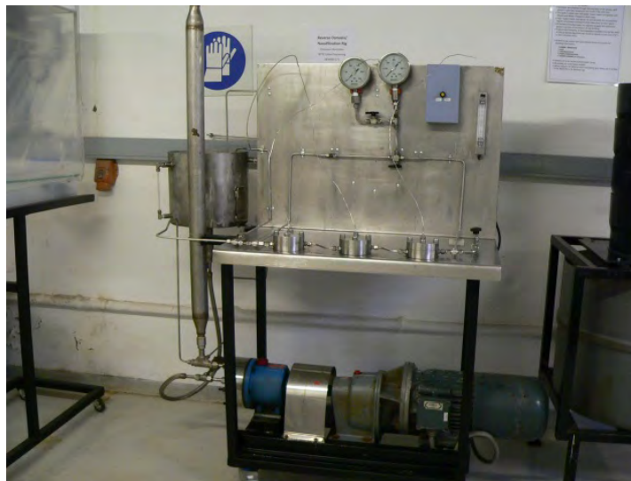
Nano Filtration Rig/ Reverse Osmosis
