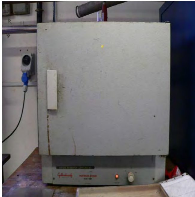
Oven (Gallenkamp) – Temperature: 105 °C
