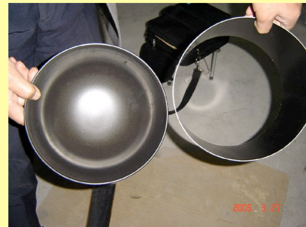
Turning bowl and install cylinder, all made of stainless steel plated with Teflon
