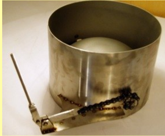
Solution 1 of turning of bowl: A rod is pushed by the lid when user seats on it to turn the bowl over for receiving the feces
