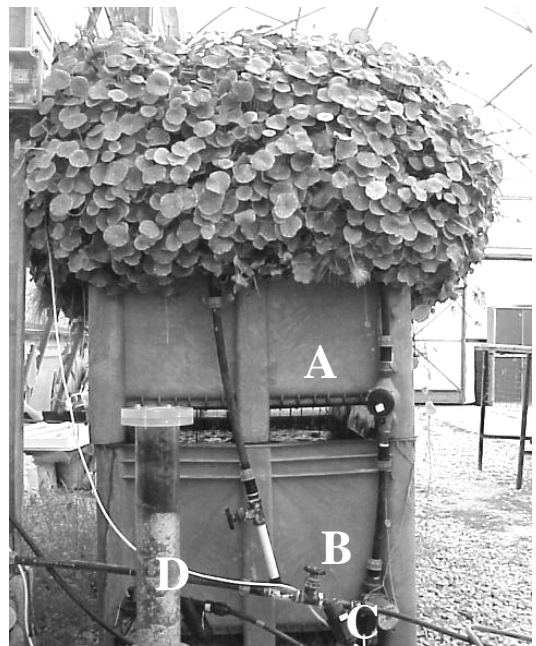
Figure 1. Recycled vertical flow constructed wetland (RVFCW). A. Wetland and Filter tank; B. Reservoir; C. Recycling pump; D. Demonstration of filter media layers (peat, tuff, and lime pebbles in top middle and bottom layers, respectively).
