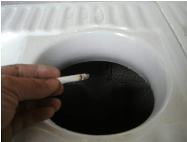
Fig. 98 : Test of ventilation-efficiency with smoke
