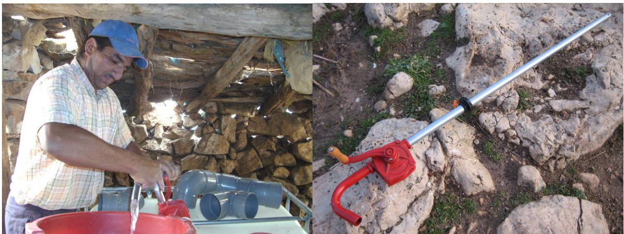
Fig. 9 : Manual Pump for emptying urine from tank [sd]
