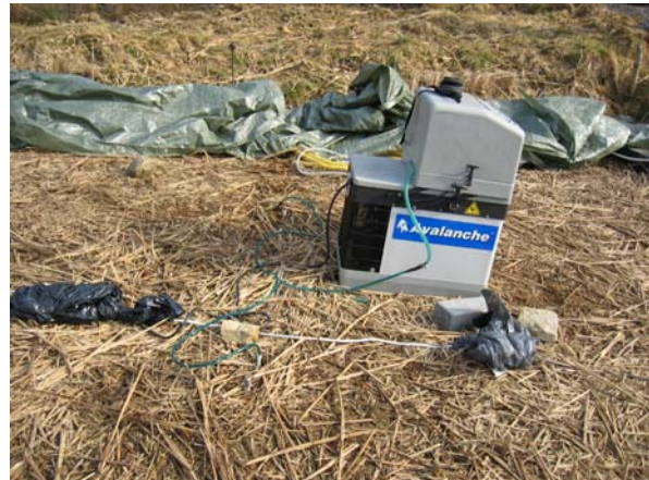
Figure 24 : Photos of the sampling layout with (left) the 3 automated samplers set on lines 1, 2 and 3 to collect the 3 investigated depths over length; (right) detail of one sampler mixing two points from the same depth located on the same transect line over length
