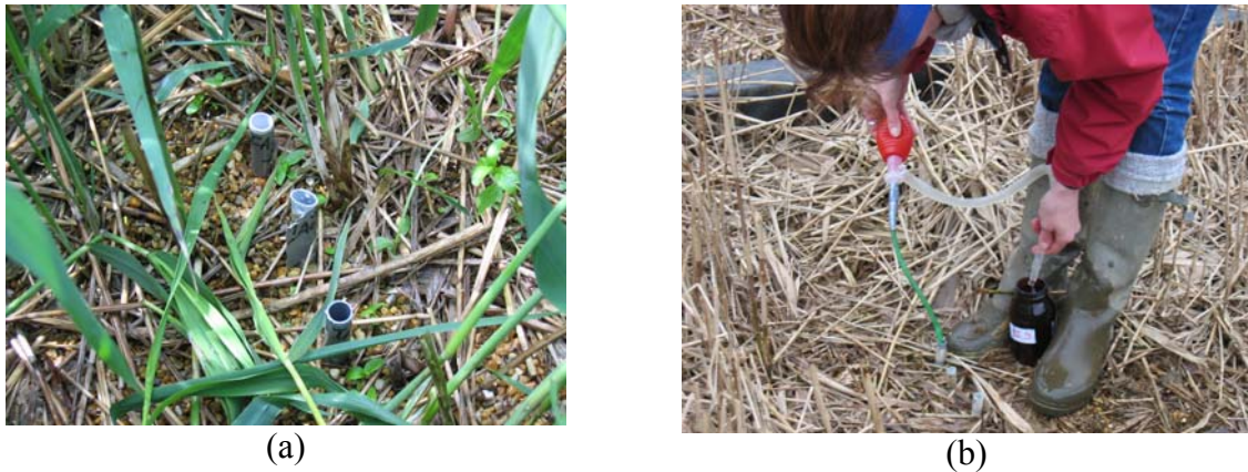
Figure 40 : Sampling ports (a) and sampling with manual vacuuming pump (b)
