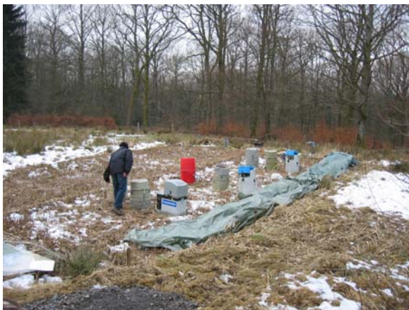
Figure 24 : Photos of the sampling layout with (left) the 3 automated samplers set on lines 1, 2 and 3 to collect the 3 investigated depths over length; (right) detail of one sampler mixing two points from the same depth located on the same transect line over length
