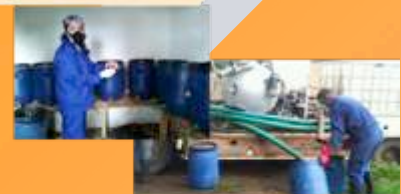
Sochi Treatment Plant: Experiment Site 50L Plastic Drum Reactors
