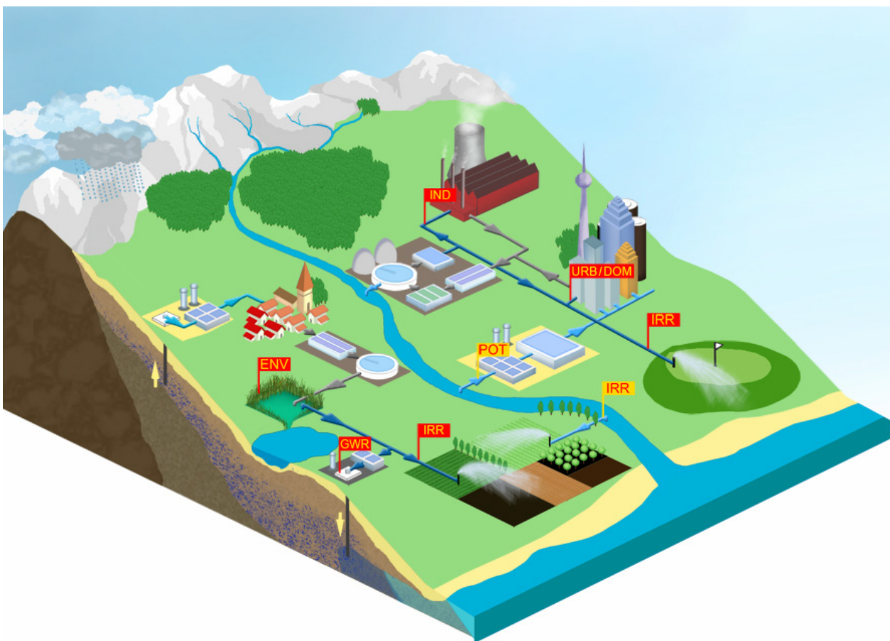
Figure 2.5: The anthropogenic water cycle with direct and indirect water reuse (modified from Veolia Water, Durham 2005, where ■ : indirect reuse ■ : direct reuse, GWR: groundwater recharge, IRR: irrigation, POT: potable reuse, IND: industrial reuse, URB / DOM: urban & domestic reuse, ENV: environmental enhancement)
