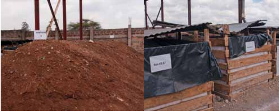
Figure 10.3 Co-compost of faecal sludge and municipal waste by Sanergy in Nairobi, Kenya (photo: Linda Strande).
