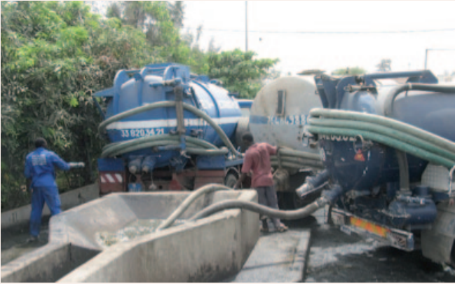
Figure 7: Delivery of mechanically emptied faecal sludge in Dakar, Senegal (picture credits to Sophie Trémolet)
