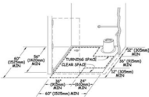
T - Turning Space in Outhouse
