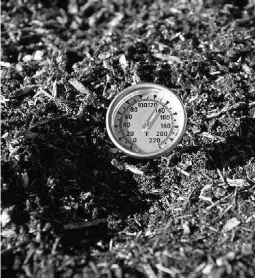
Figure 1. Probe to measure compost temperature (Fahrenheit).
