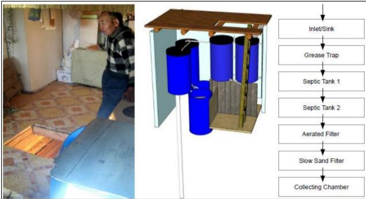
Figure 26: Photo of the location (left), flow chart (right) and model of the UGTU built in 2010 (ACF, 2012; modified by Schüssler, 2010).
