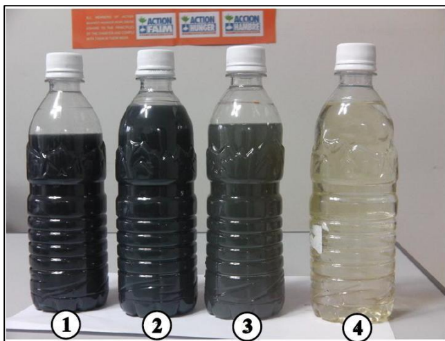
Figure 35: Visual analysis of greywater from the GHTU. Samples taken 1.5 weeks after filling up of the system and after each of the four treatment steps (ACF, 2013).
