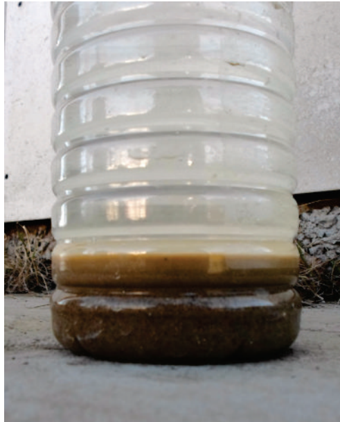
Picture A: Sand layers of different grain size in a water bottle.
