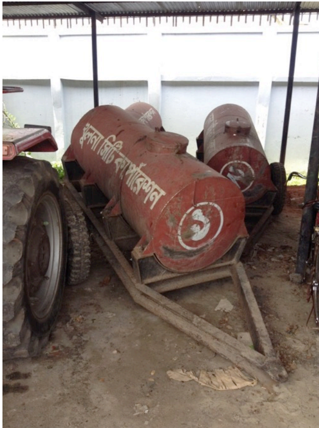
Figure 6: A 1 m 3 towable bogey that is no longer in operation. Photo: Arief Gunawan
