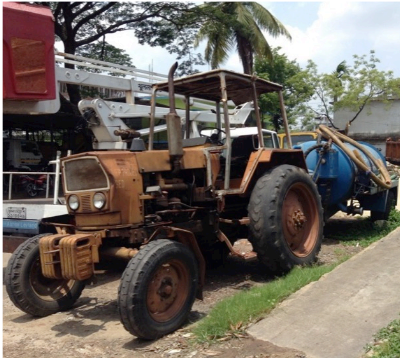
Figure 5: Tractor with 5 m 3 container tank used for motorized emptying services. Photo: Arief Gunawan
