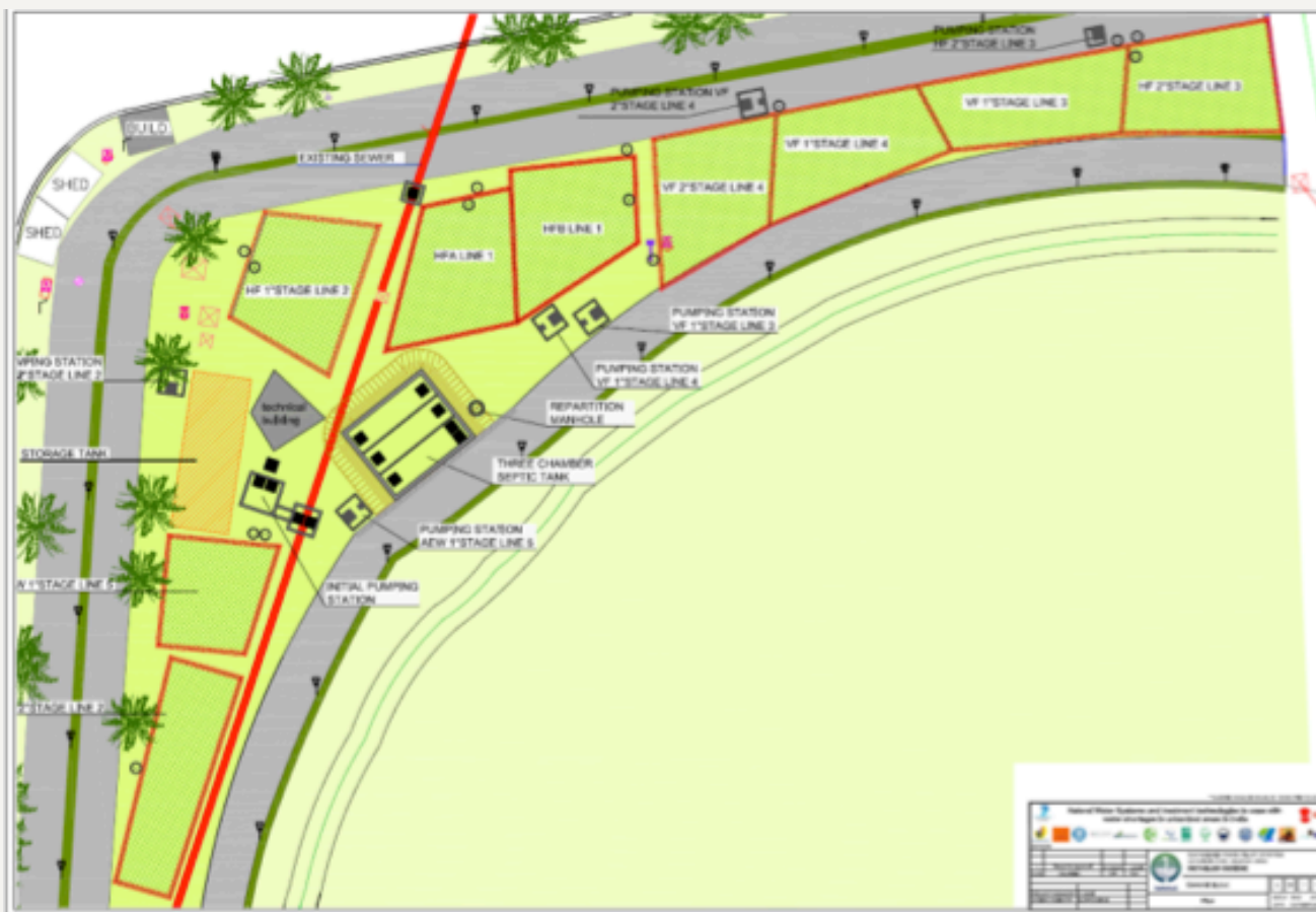
Figure 1: Schematic of the treatment system (source: Iridra and Kreta, 2014)
