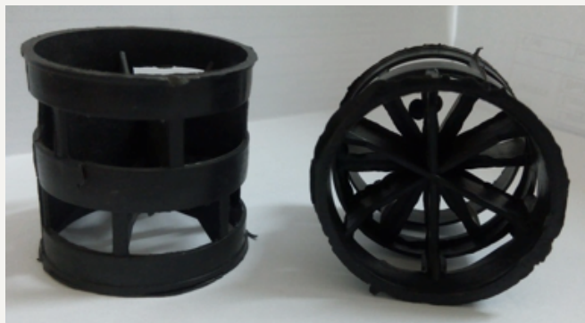
Figure 2: Anaerobic filter media (Pall rings) made of PP/HDPE featuring high specific surface area 150 – 200 m 2 /m 3
