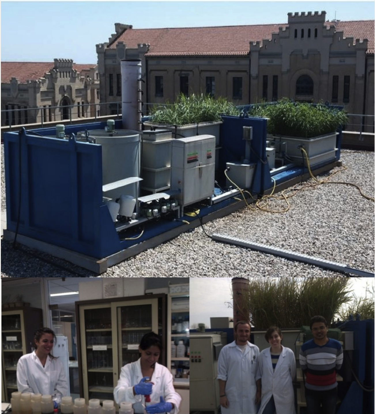
Figure 2. View of the three-stage hybrid constructed wetland system and some of the students involved in the monitoring of the system
