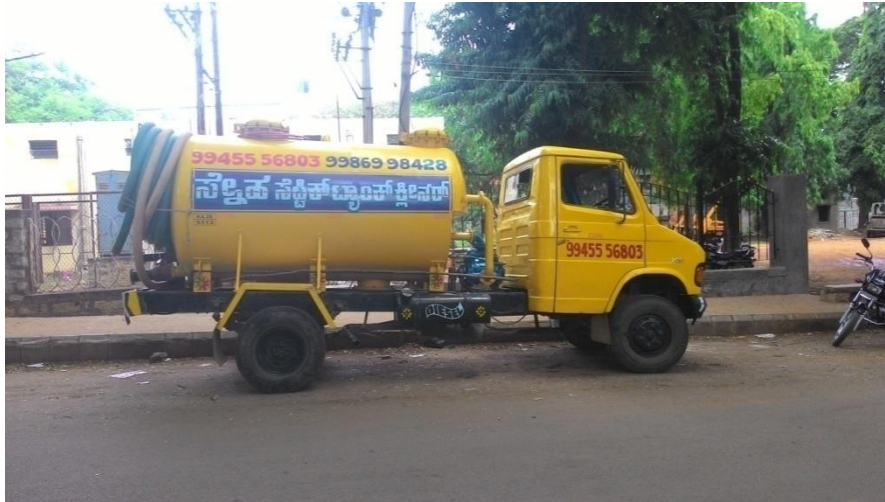
Figure 3: A Private vacuum tanker parked in municipal premises (Source: Rahul/CSE, 2015)
