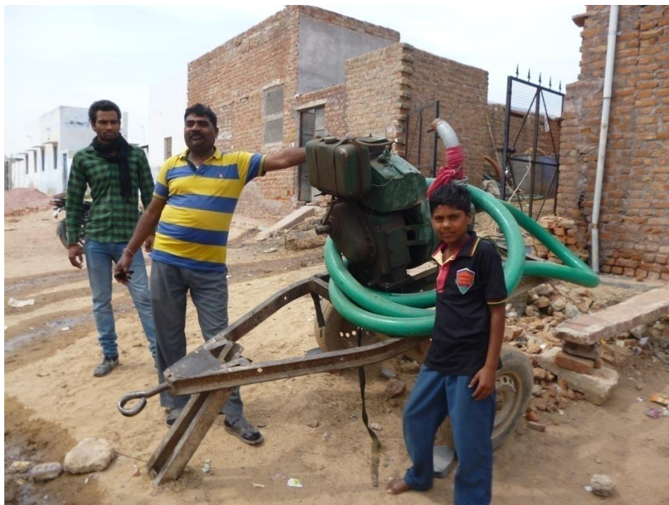
Figure 7: Generator based suction pump (Source: Rahul/CSE, 2015)
