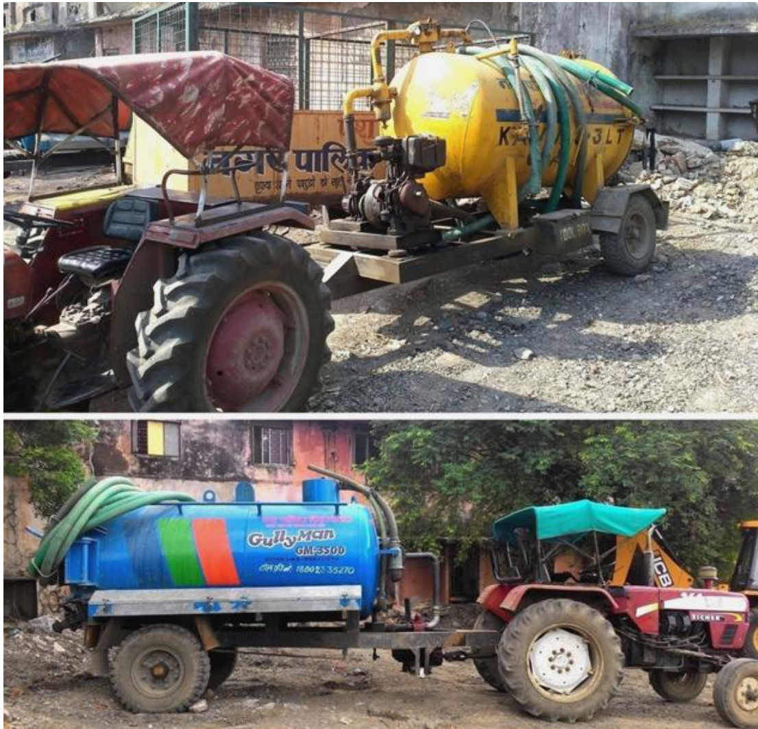
Figure 8: DMC vacuum tankers used for emptying septic tanks/pits (Source: Anil/CSE, 2015)
