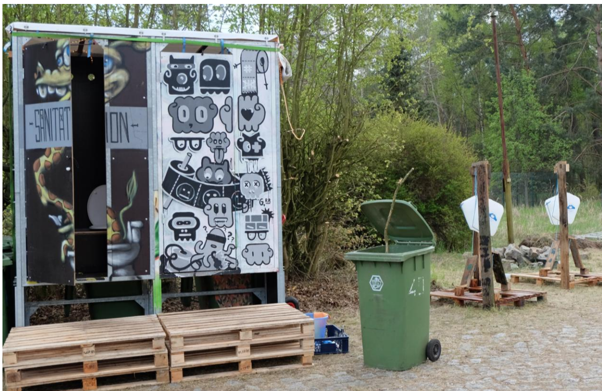
Image 2: Metal framed Goldeimer toilet cabins with sawdust container and tippy taps aside, © Goldeimer
