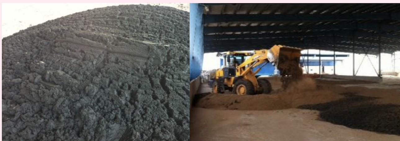
Figure 3. WWT sludge and mixing process
