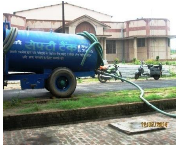
Vacuum Truck for desludging
