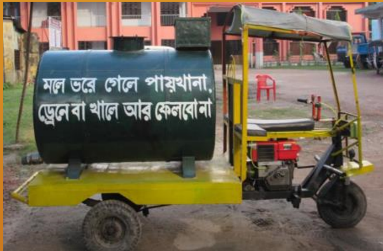
Low-cost locally fabricated of capacity 1000 liters & cost 1500 USD
