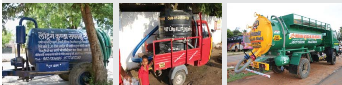
Fig. 26 : Variety of mechanical modes to desludge septic tanks
