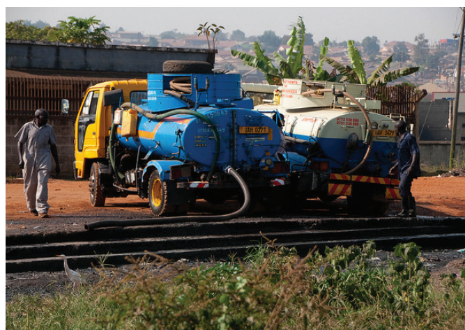
Trucks emptying faecal sludge at Bugolobi Wastewater Treatment Plant in Kampala, Uganda.
