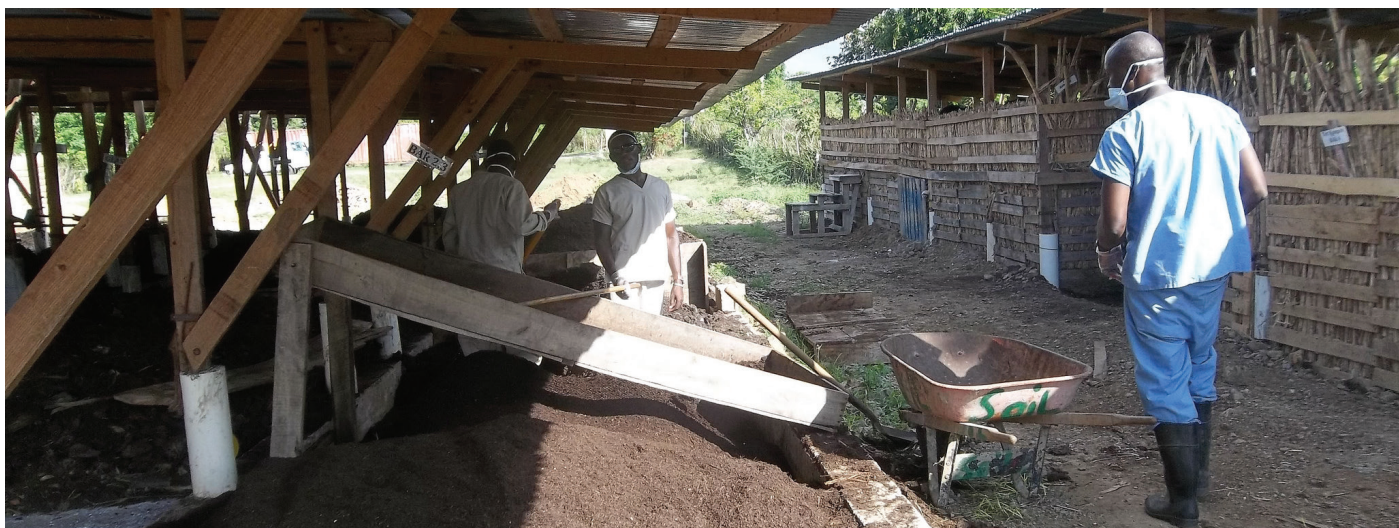
Sieving compost made from excreta and organic solid waste, in preparation for sale at a facility operated by SOIL Haiti
