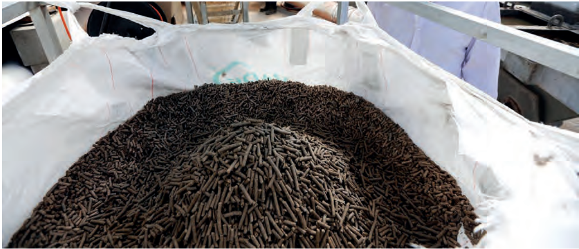
Pellets of cellulose fibre recovered from sewage. These pellets, marketed under the name Recylose, can be used as fuel or in producing paper, insulation, construction materials and bioplastics. Photo: Reuters / Baz Ratner
