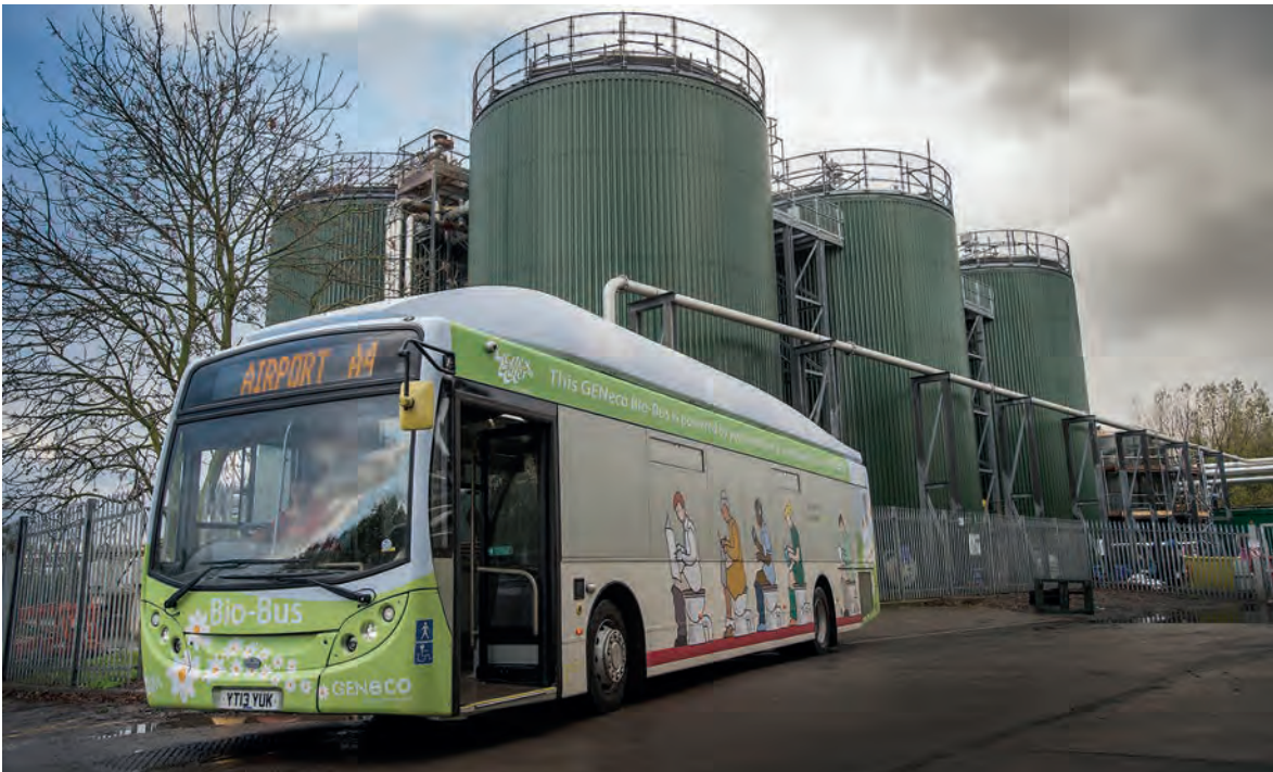
The Bio-Bus, running on biogas produced at a centralized sewage treatment plant, UK. Photo: Wessex Water
