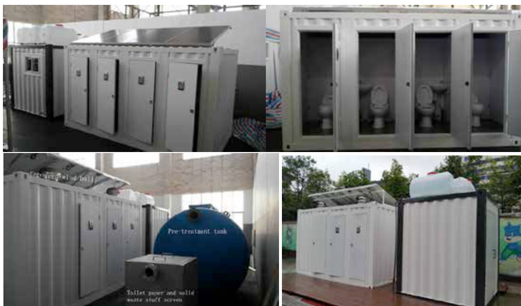
Figure 2. Beta prototype PV-powered solar toilet system used at an elementary school in Yixing, China.
