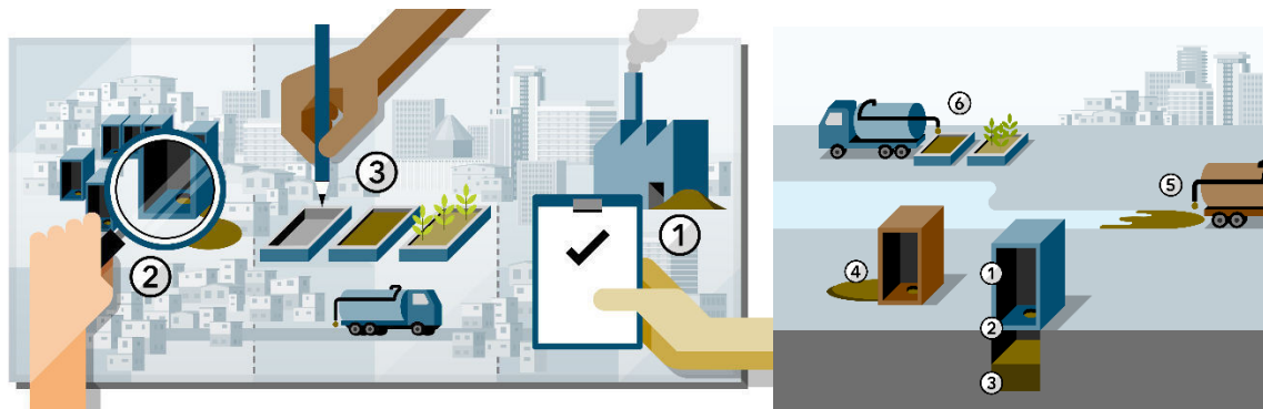
Figure 1: Left – Schematic of Engineering Design Approach, including: 1) Treatment Objectives and Resource Recovery; 2) Faecal Sludge Quantification and Characterization; and 3) Treatment Technologies for Resource Recovery. Right – Schematic of Quantification and Characterization, including: 1) excreta produced; 2) FS produced; 3) FS accumulated; 4) FS emptied (but not collected); 5) FS collected (but not delivered to legal discharge); and 6) FS delivered to legal discharge.
