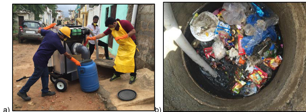
Figure 1 a) The Flexcrevator unit in Hyderabad, India b) example of a pit with high trash content.
