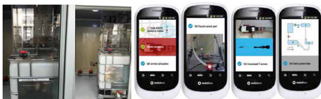
Figure 3. Left Panel: Alpha prototype showing the electrochemical reactor arrays, the baffled anaerobic reactor, flush water tank, and the biochemical reactor effluent holding tank. Right: Smartphone monitoring and control systems for operational control, maintenance, and repair directions.
