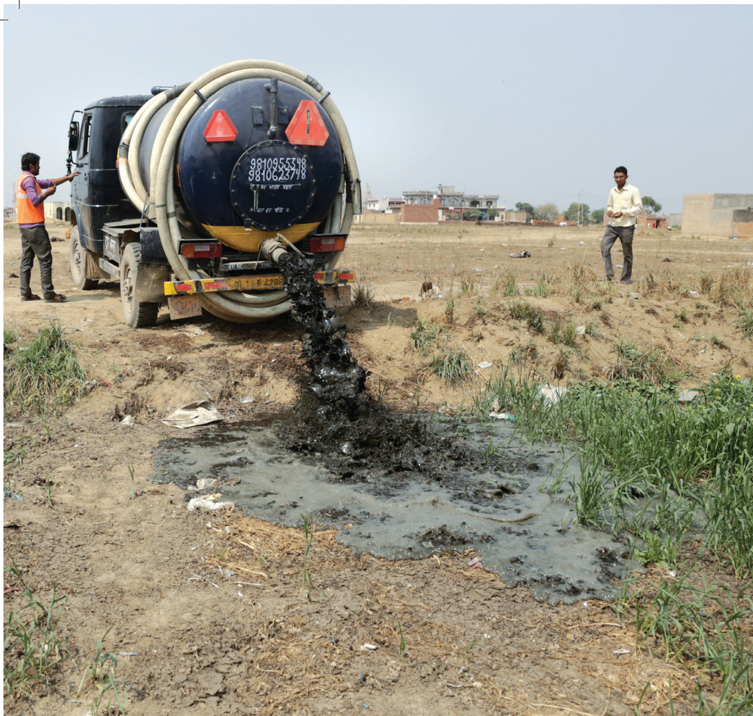
A vacuum tanker dumps untreated faecal sludge in a wheat field in the National Capital Region
