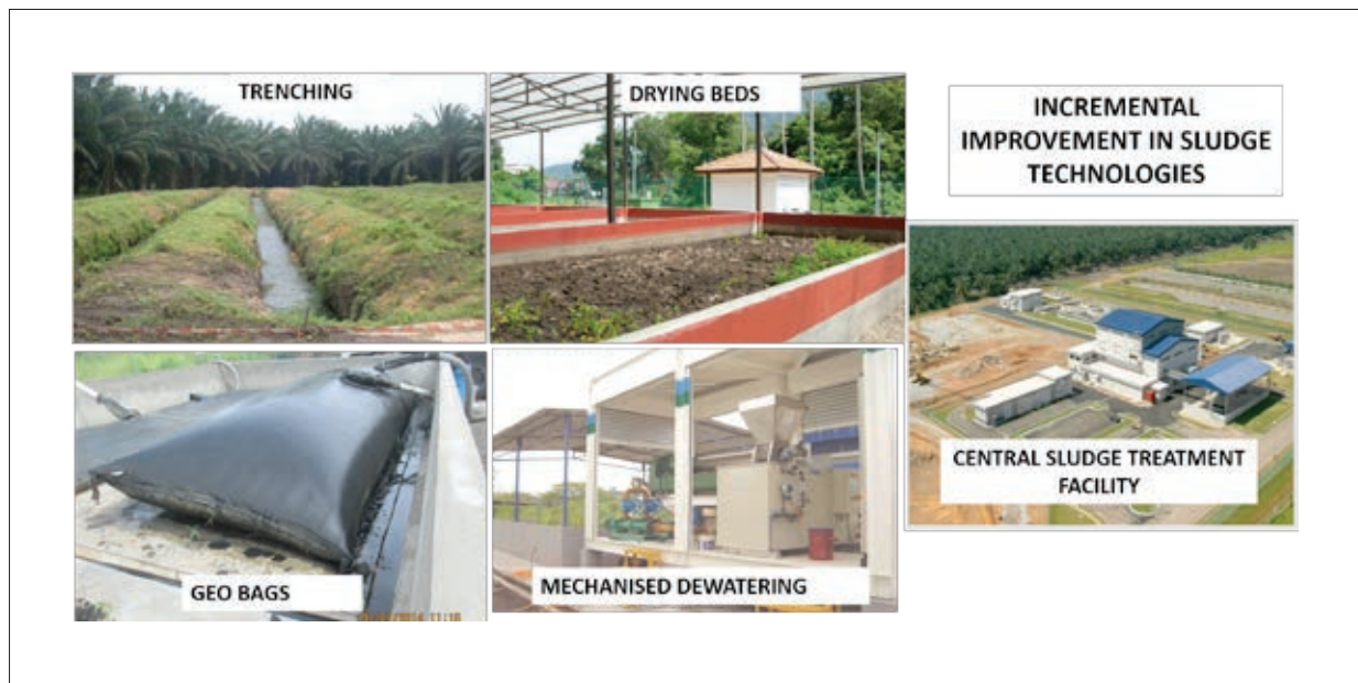
Figure 2: Improvements in Sludge Treatment Technologies
