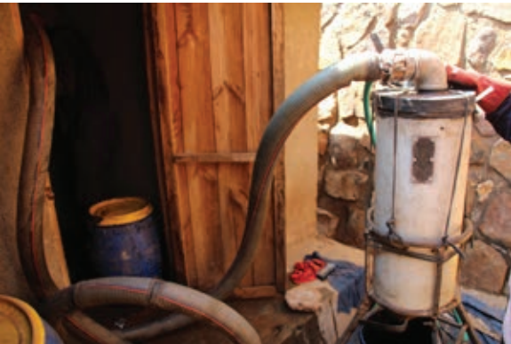
Figure 4. Modified eVac designed to reduce splashing and labor requirements.
