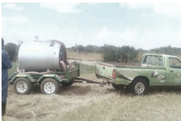
Figure 4: Mobile Desludging Units (MDU) in Norton
