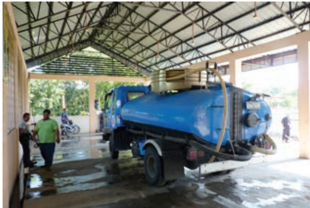
Figure 5a: Motor pool building installed in 2012 to better maintain the trucks. 5.b: Fleet mechanic inspects old desludging truck tank. To keep costs down, vacuum tanks are now fabricated on site.
