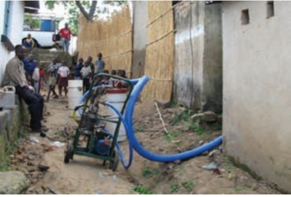
Figure 3. eVac in a Narrow Alleyway. (Figure from eVac User Manual (2015), PID Consulting Engineers and Project Managers)
