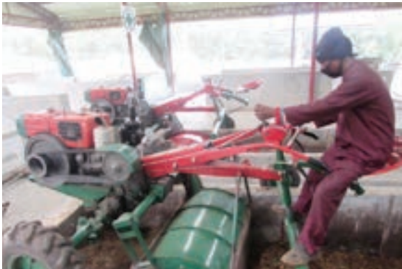
Figure 12: Sludge turner in Sakhipur
