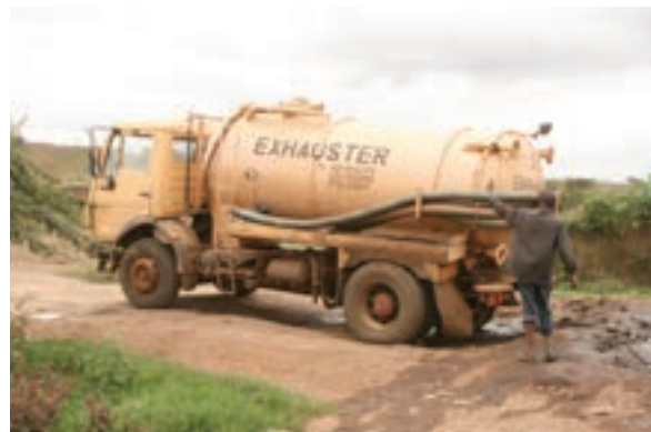
Figure 4: Private vacuum truck at a designated discharge point ©GIZ/Cees Lafeber
