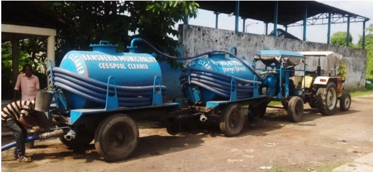
Figure 5: Tractor mounted vacuum tanker (Source: Anil/CSE, 2016)
