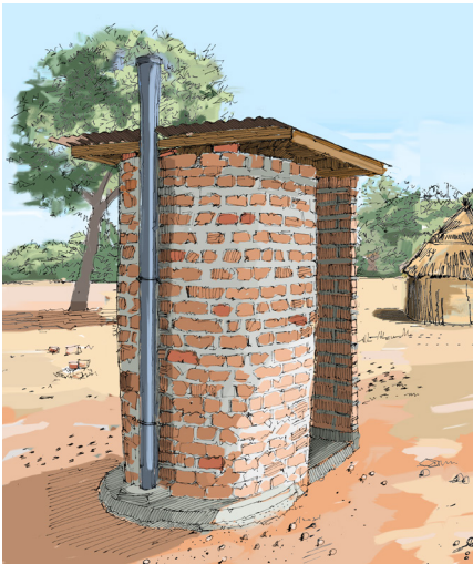
Figure 2. Original spiral designs had no door to maximise the air flow throughout the latrine (a). However, many users were concerned about privacy and safety so half doors have been added still allowing a sufficient flow of air whilst controlling access to other users and animals (b). Figure 3 shows the internal layouts of typical spiral designs.
