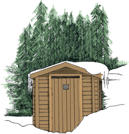
Figure 7. A lightweight structure will warm up quickly during the day
