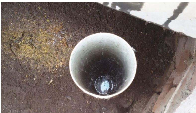
Figure 4 Inside the tank after 12 months; the photo also shows the sample collection pipe
