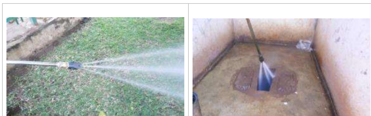
Figure 9. Spray pattern fluidizer using a 4 jet nozzle at 100 bar
