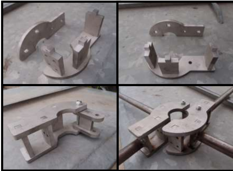
Figure 21: Example of a ‘puzzle’ for cutting cost in production
