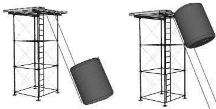
Figure 54: Sketch of suggested method on how to lift the water tank.
