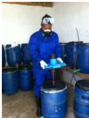
Figure 13: a) Mixing Faecal Sludge with Hydrated Lime. b) 50L reactors
