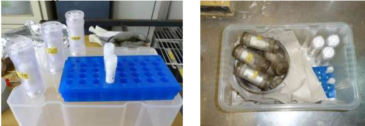
Figure 15: Germ carriers before and after heat treatment in pasteurizer plus control samples
