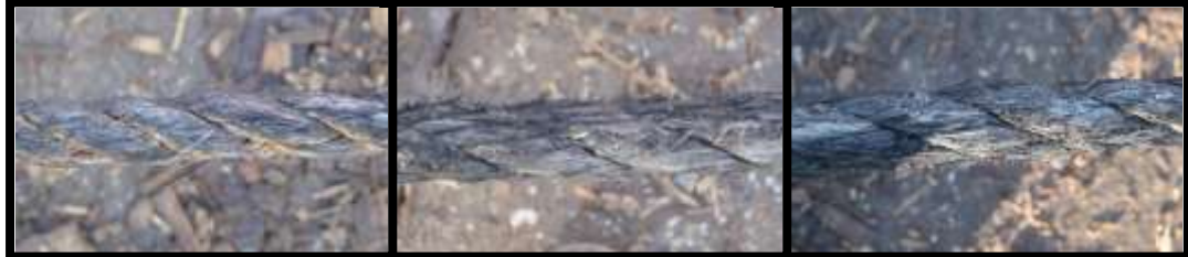
Figure 23: Manilla rope: left picture 2 wraps, 76 kg, 80 rpm, middle: 2 wraps, 118 kg, right: 80 rpm/2 wraps, 160 kg, 80 rpm
