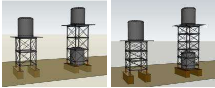
Figure 49: Impression of rectangular tower structures of 3m and 5m height built with modules of 1,5m (left) and 1m (right).
