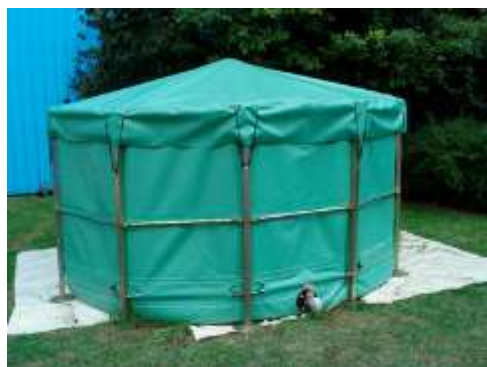
Figure 27: 10m 3 steel frame reservoir.
