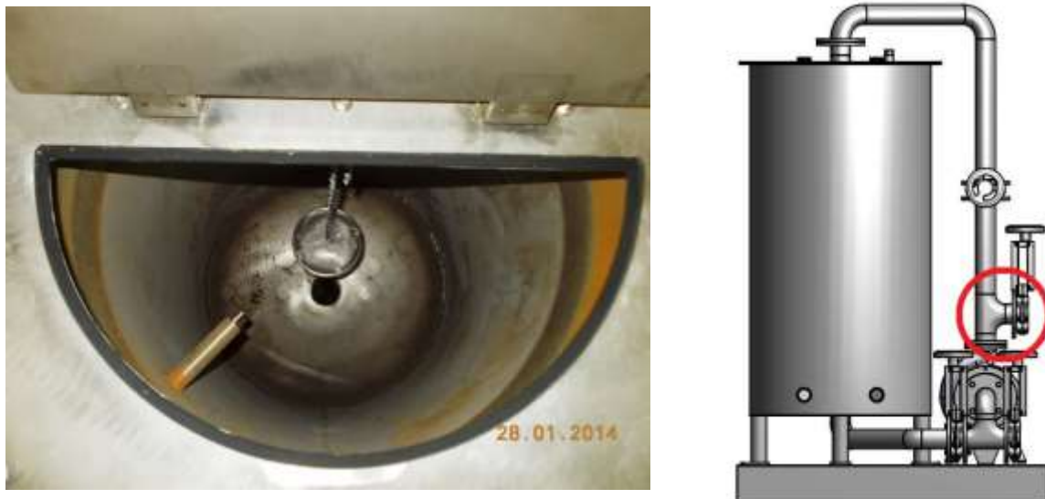
Figure 16: Test points in pasteuriser (left: tea ball on chain in main vessel, right: tea egg at valve in pipeline)
