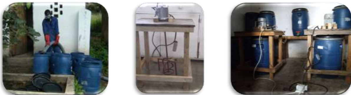
Figure 11: filling the drums (left); one of the two custom made mixers (middle); overall set-up (right)
