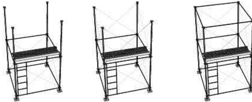
Figure 53: Illustration of three steps in the proposed assembly method using a temporary platform.
