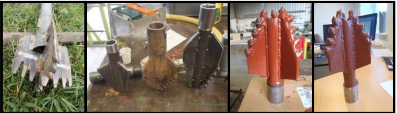
Figure 18: Evolution of drill bit design
