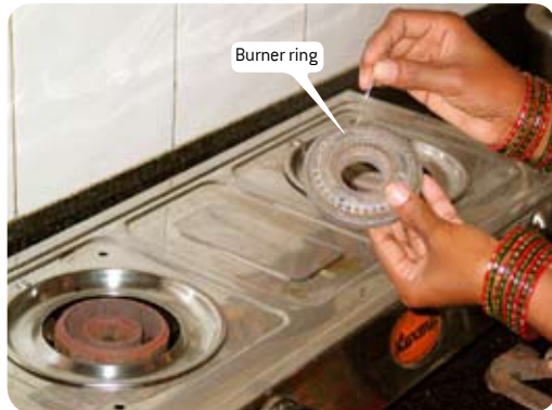
Cleaning of burner ring holes
